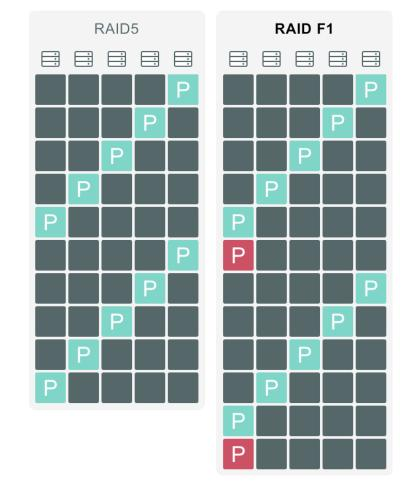
Since each write-operation involves writing to the parity block, it is expected that the parity block will be worn out in the first place. This uneven parity distribution approach will lead to that one SSD reaches its lifespan earlier than others, instead of making all SSDs reach the end of their lifespan at the same time. When one SSD fails, the customer can replace it with a new one.
