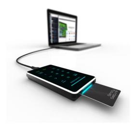
Insert the smart card into the smart card slot with the contacts facing up.
